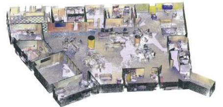
Color point cloud of commercial office space – note detail of wall colors and flooring
